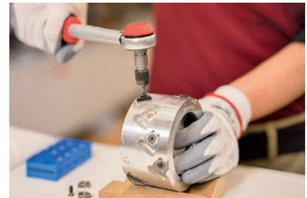
WhisperCut: Diamond knives are resharpenable in the tool body up to 3 times
